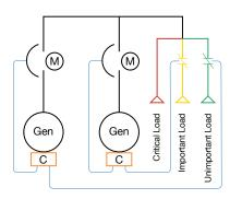
Parallel Generators with Load Management in Controller
