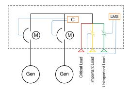
Parallel Generators with Load Management System (LMS)
